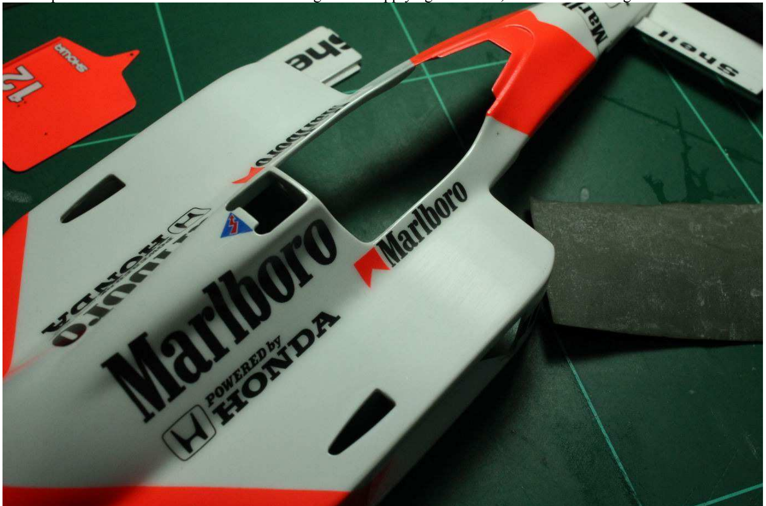
20. Sanding the surface after the clear coating is dried hard enough.
