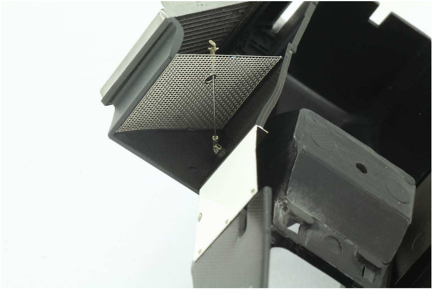
59. A mesh added on both air intakes.
