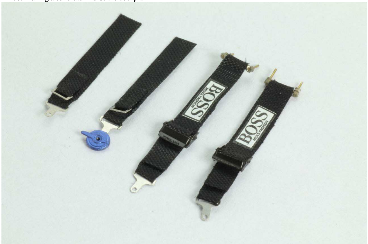
78. Making the seat belt with and fabric, PE buckle and small metal bar.
