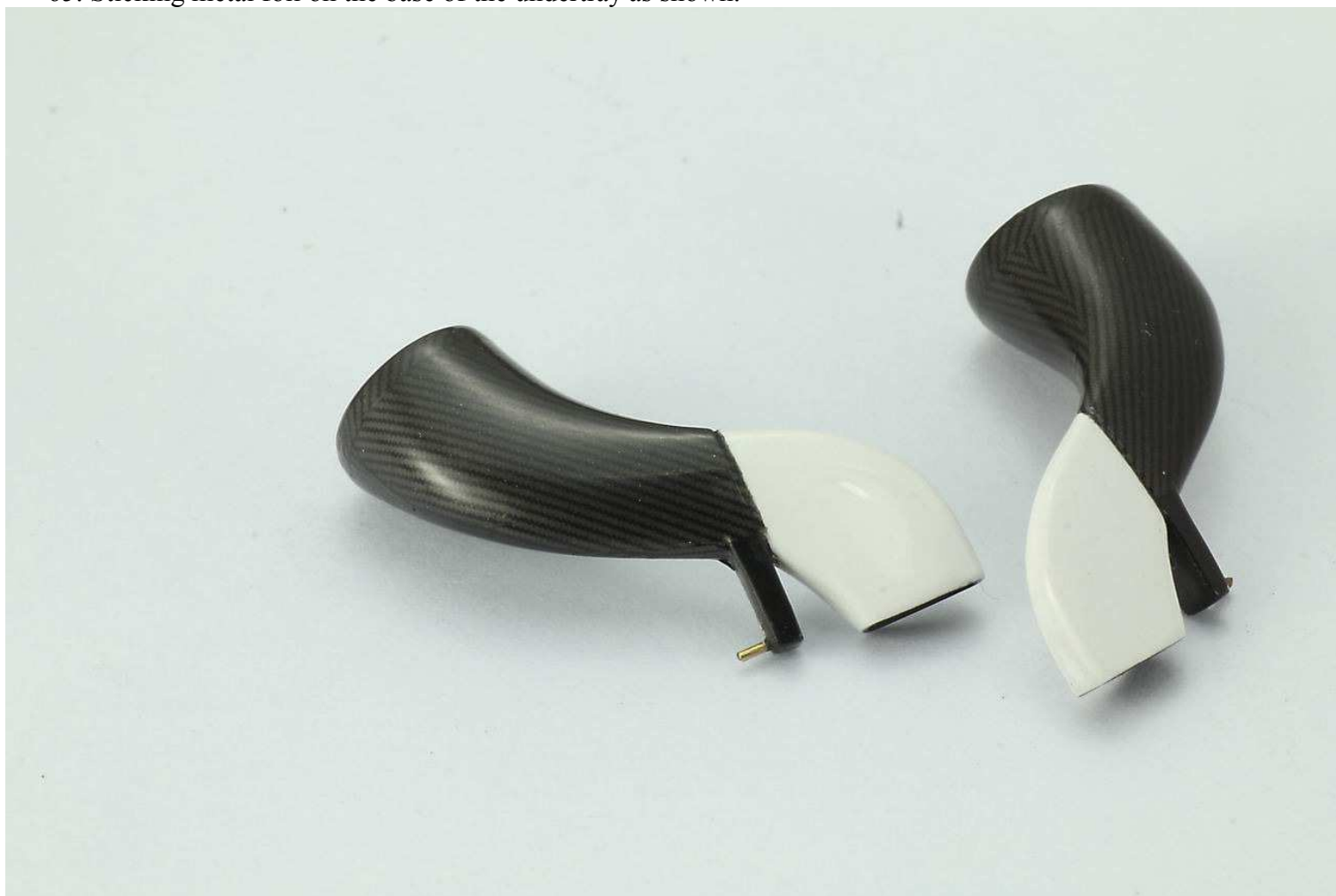
66. Applied carbon fiber decals on the upper part for the turbo air intakes, with a few coats of smoke paint sprayed.
