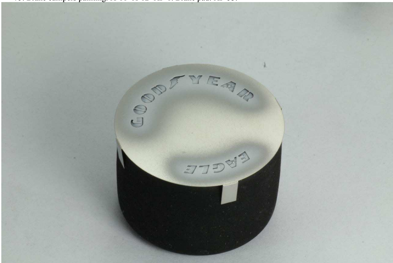
76. Painting the tyre marking with the help of the PE template. Spraying with light grey then white.
