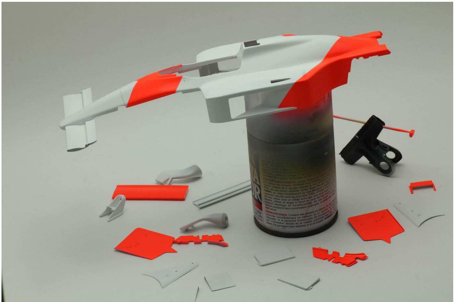
19. Body painting: white first then fluorescent red. The fluorescent red paint is mixed with some clear gloss to prevent fluorescent color surface cracking. Before applying the decals, a thin clear coating is a must.
