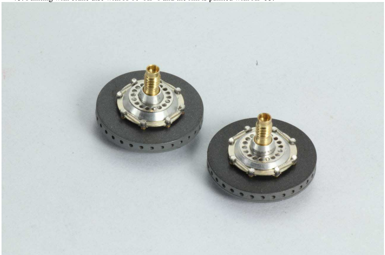
74. Putting the previous made central part and axle to the brake disc.
