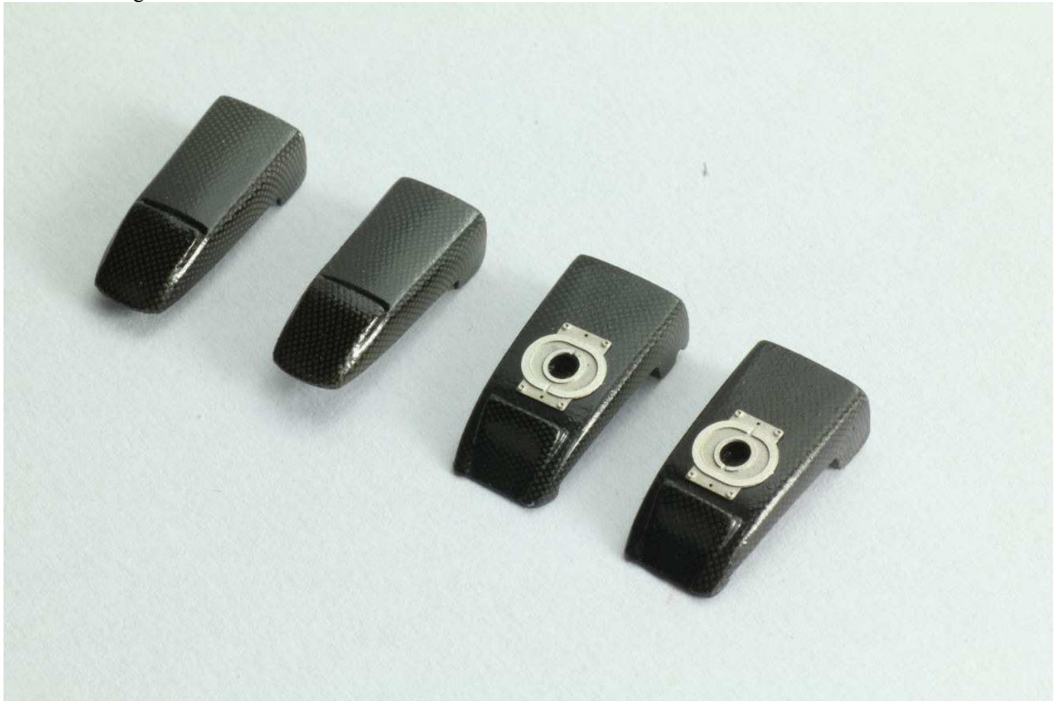
84. The carbon fiber effect of the brake disc air ducts is made by spraying over a mesh.
