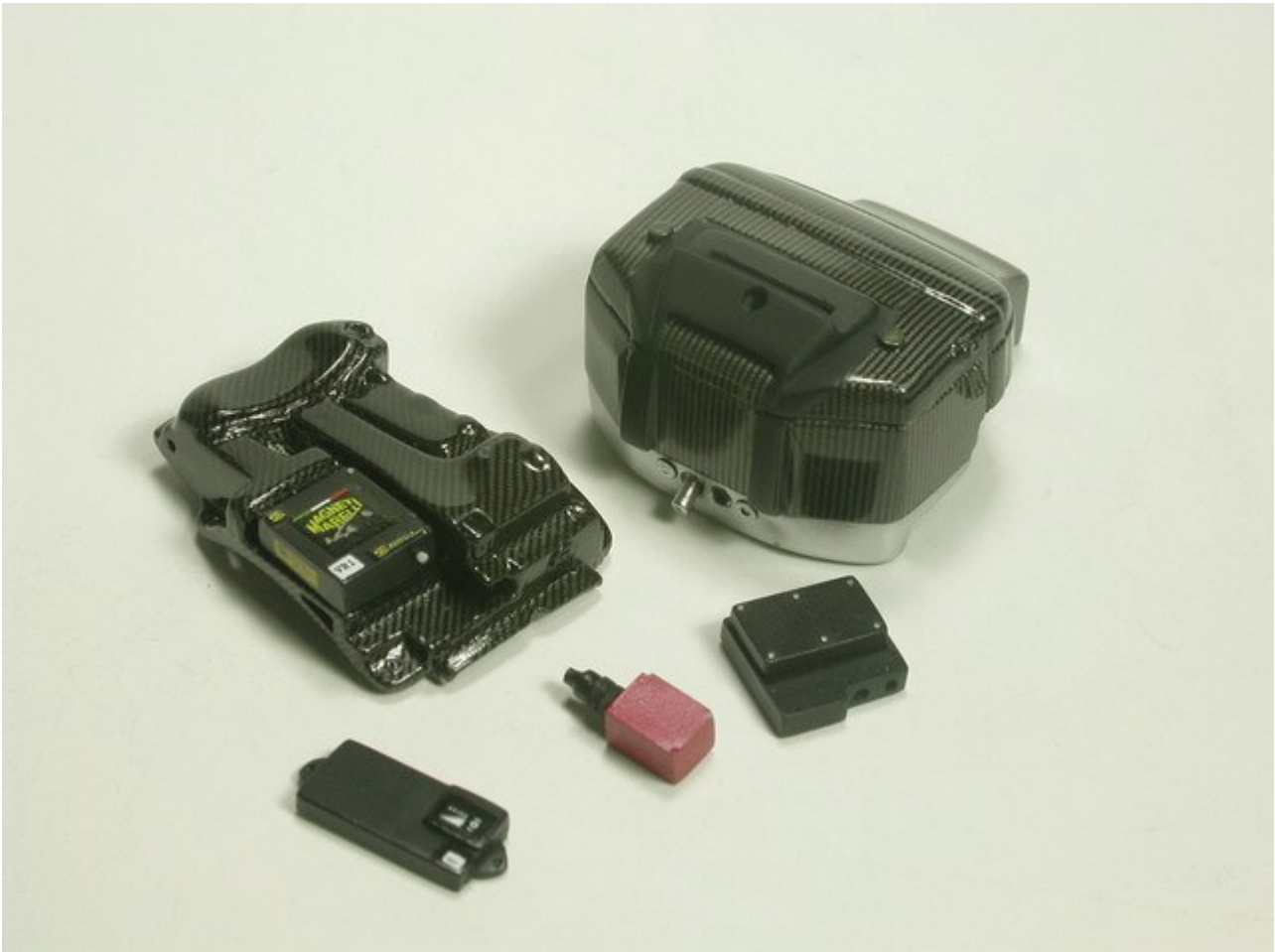
29. Airbox, electronic boxes and related parts are painted and carbon fibered.
