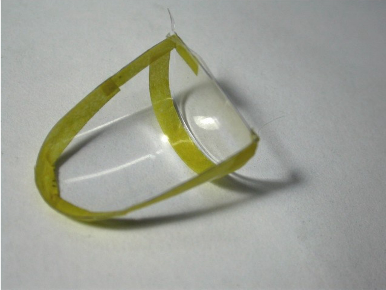
9. Wrapping around the edge of windscreen with masking tape as trimming line.
