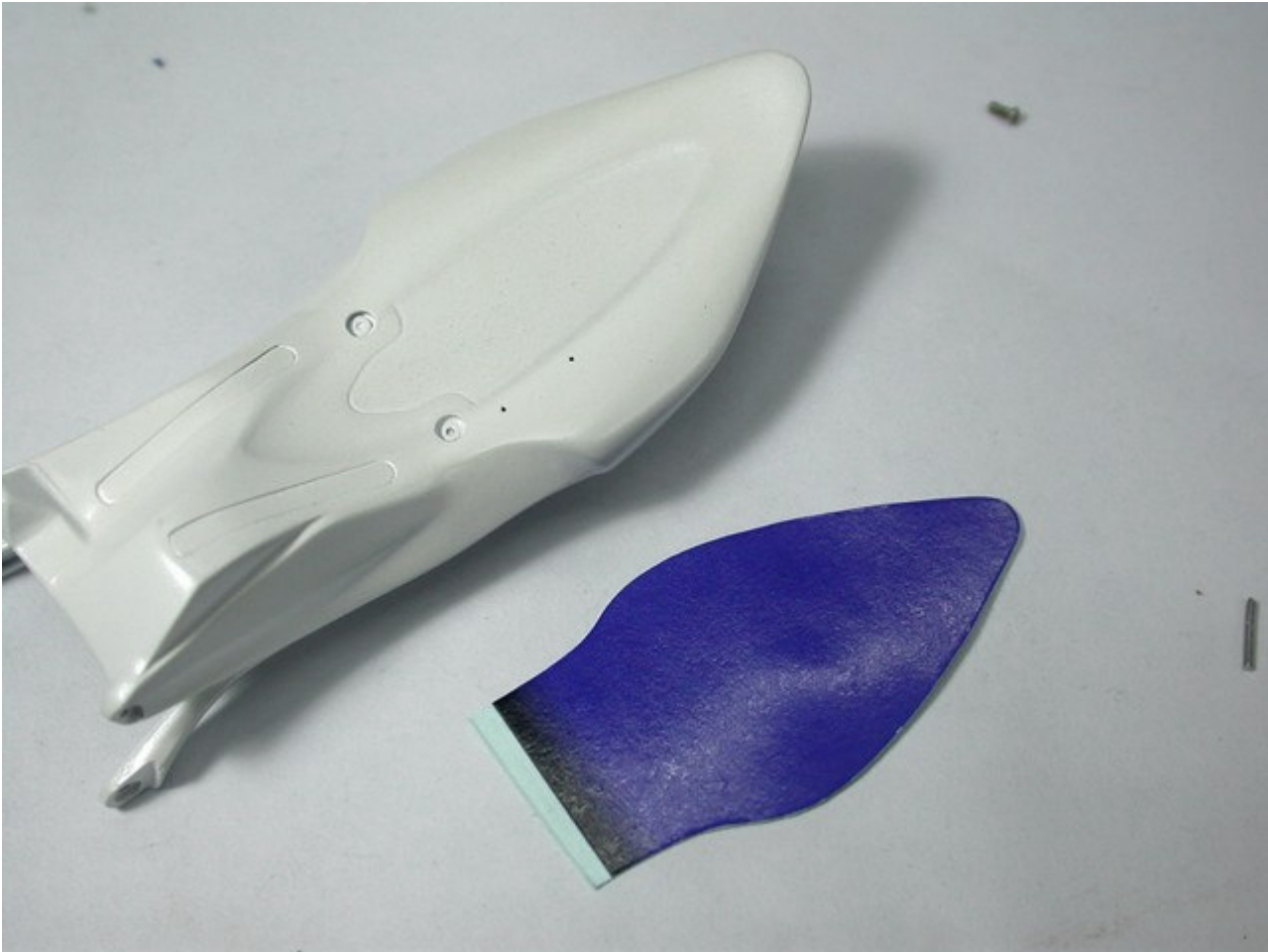
13. Applied the painted decals and masked the area for carbon fiber.
