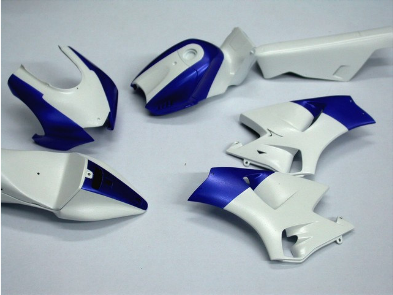
6. With mica blue paint applied.
