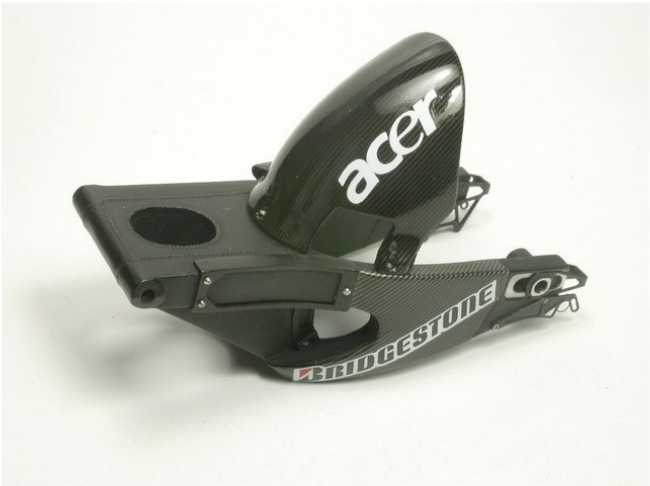
22. Rear fender fitted on top of the swingarm.
